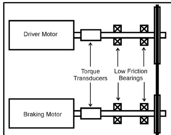
Figure 1: Drawing of a test bench measuring chain drive efficiency [1].
