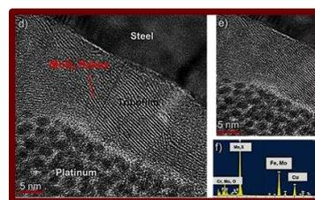
Figure 1: FIB-TEM images of tribofilm (flat) obtained under boundary lubrication with MoDTC [A] after 250 cycles.
