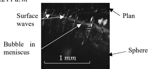
Figure 1: Lateral view of the rear of an EHL contact with the highlighting of bubbles in the liquid lubricant for  $\eta \cdot u_e = 1.24 Pa \cdot m$
