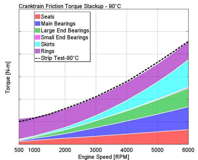
Figure 1: Overall cranktrain system friction torque (stacked) compared with measured strip down data.
