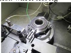
Figure 2: Wheel bearing on friction functional test bench
