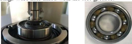
Figure 1: Rolling Bearing Assembly system on MCR502S rheometer used for grease flow behavior study
