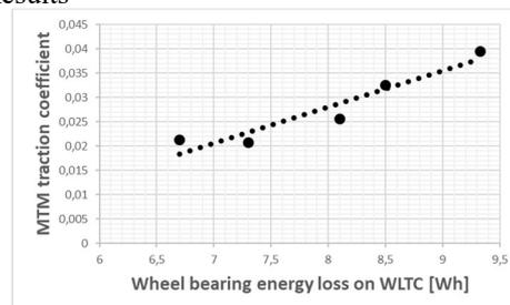
Figure 3: Good correlation between entire wheel energy loss on WLTC and MTM traction coefficient at 40°C
