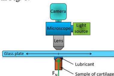
Figure 1: Scheme of the experimental apparatus.
