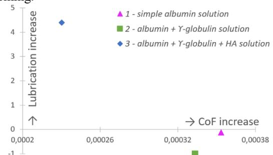
Figure 2: Dependency of lubricant composition on lubrication and friction of albumin protein
