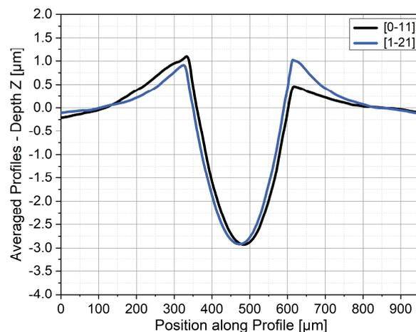
Figure 1: Anisotropic average wear track profile for sliding in [0-11] direction as opposed to [1-21] direction on a (111) single crystal
