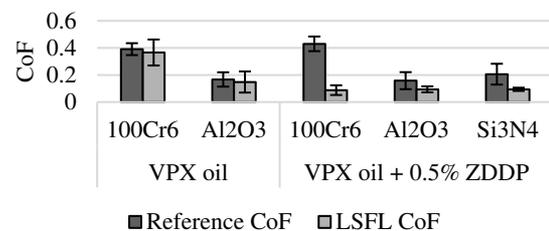
Figure 1: Mean values and standard deviations of the coefficient of friction (CoF) corresponding to the entire RSTT.
