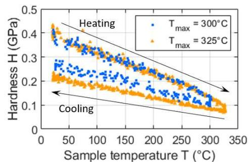
Figure 1: Hardness vs temperature for tested pure aluminum samples during 3°C/min thermal ramp cycles.
