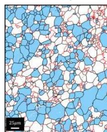
Figure 2: Microstructure of one of the studied aluminum samples after the thermal cycle up to 325°C, obtained by EBSD measurements (black: grains boundaries, red: sub-grains boundaries, blue: recrystallized grains). Recrystallization clearly occurred during the thermal cycle.
