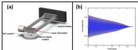
Figure 1: Dynamic oscillating tribometer measurement
