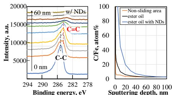
Figure 2: XPS depth profiles of the specimens
