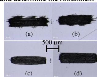
Figure 1: Wear tracks generated for the critical assessment of the wear volume determination methods.
