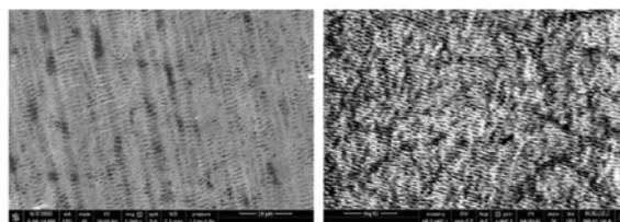
Figure 1: SEM images of the LIPSS on TiN (left) and on TiCN showing a more pronounced structure (right).
