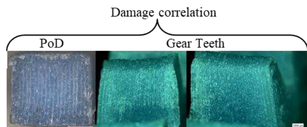
Figure 1: Comparison of the damage of running surfaces from pins (32x magnification) and gear teeth (10x magnification).
