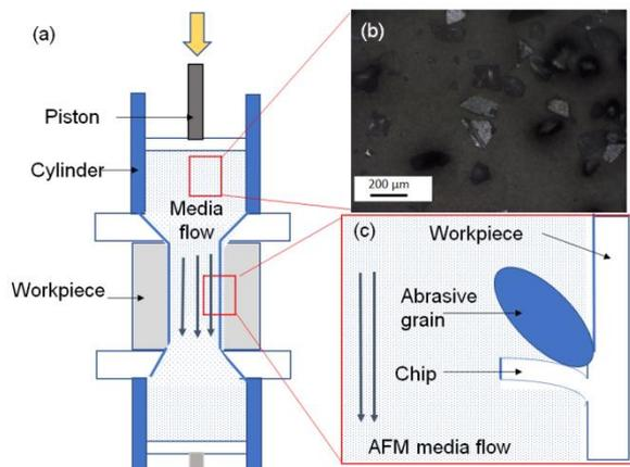
Figure 1: Schematic illustration of AFM process in an internal channel of a workpiece [1].
