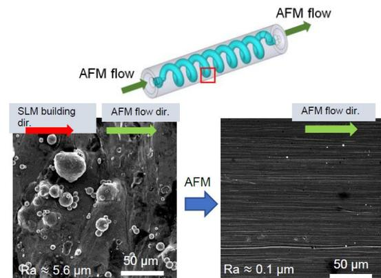
Figure 2: Surface topography evolution of SLM conformal channels with AFM [2][3].
