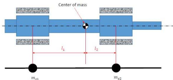
**Fig. 1** Scheme of the equivalent lumped masses spindle.
