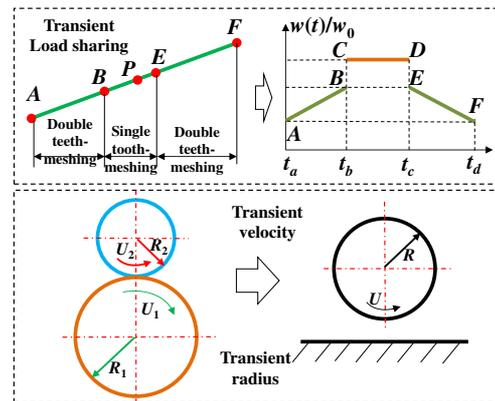
Fig.1 Transient-load sharing, curvature and velocity
