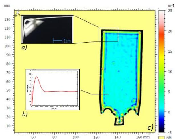
Figure 1: a) framing effect picture, b) typical framing effect profile, c) deflectometric curvature map
