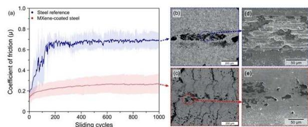
Figure 1: Tribological evaluation of the MXene coatings compared to an uncoated reference. (a) evolution of the COF. SEM micrographs of the worn surfaces for (b,d) the reference and (c,e) the MXene-coated sample.
