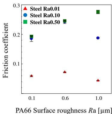
Fig. 1 Friction coefficient of PA66 vs. steel at a load of 300 N
