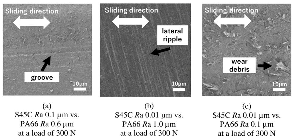
Fig. 2 SEM images of worn PA66 surface
