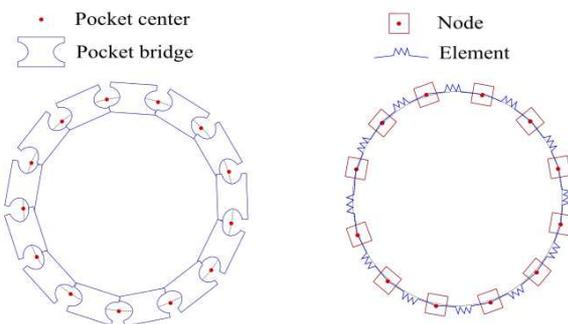
Figure 1: Finite Element cage discretization.
