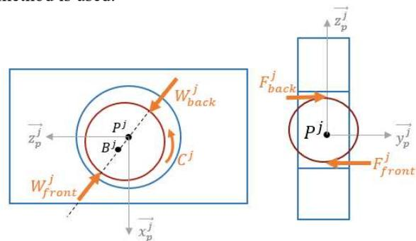
Figure 2: Ball-to-cage pocket interactions.
