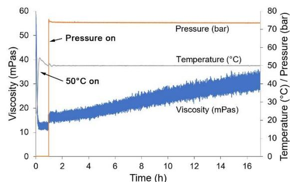
Figure 1: Example of ionic liquid viscosity changes due to gas absorption.
