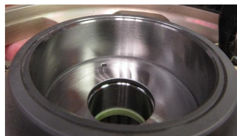
Figure 2: New Bearing liner after test
