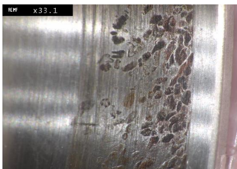
Figure 1: Galling on a bearing liner in MRO
