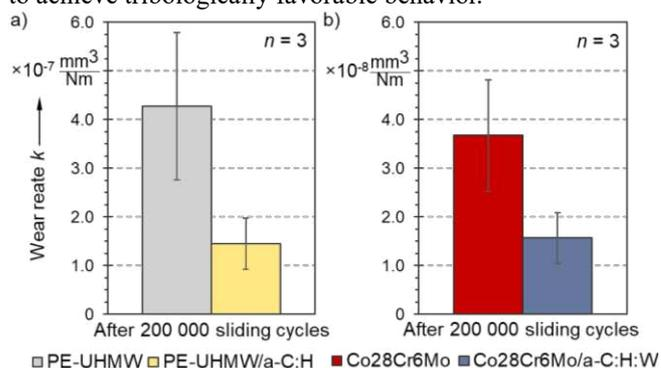
Figure 1: Arithmetic mean and standard deviation of wear rate of PE disks (a) and CoCrMo pins (b).
