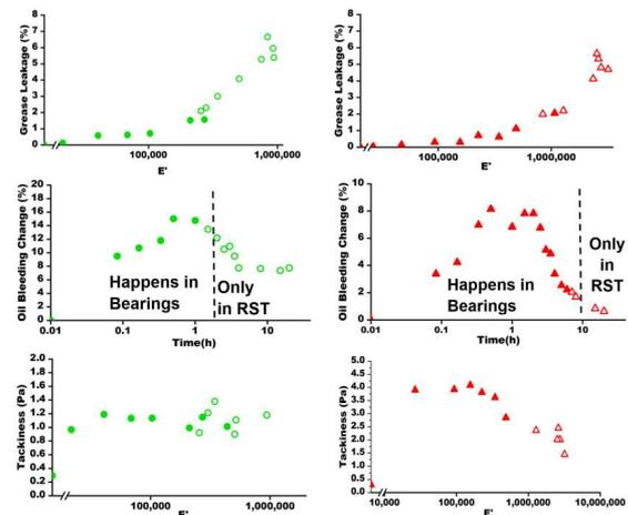
Figure 1: Grease properties. Good/peak-type (green markers) and Poor/plateau-type (red markers)
