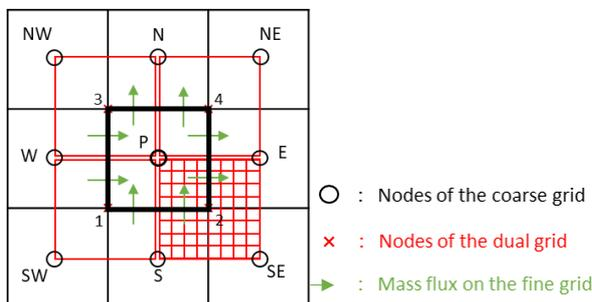
Figure 1: Coarse, dual and fine grid discretization
