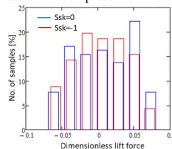
Figure 3: Lift force variation with roughness skewness
