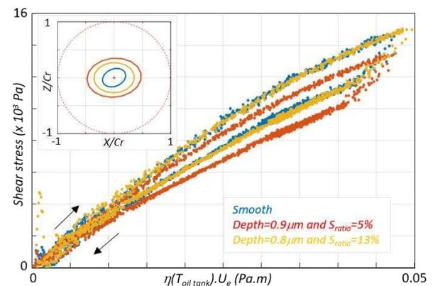
Figure 1: Illustration of the shear stress evolution vs entrainment product, viscosity\*velocity, for smooth and textured shafts (depth of 0.9  $\mu\text{m}$ , dimple densities of 5% and 13%). The dimensionless shaft center position, corresponding to the film thickness distribution (clearance  $Cr$  of about 5  $\mu\text{m}$ ), was also indicated in the inset.
