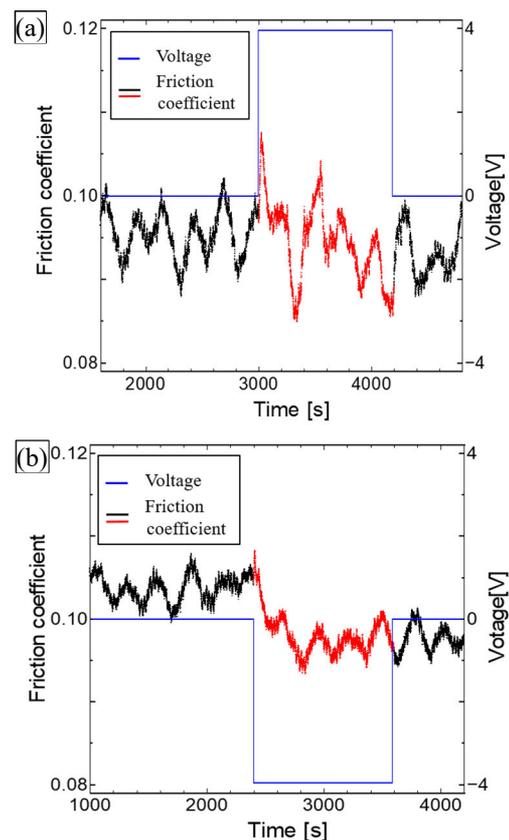
Fig. 1 friction behavior depend on applied potential (a) +4.0 V, (b) -4.0V
