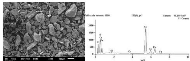
Figure 1. SEM morphology and EDX analysis of the Fe-Cr-C powder.
