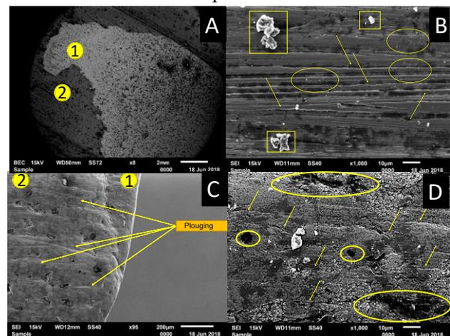
Figure 2. Wear mechanisms in the subsoil rod.
