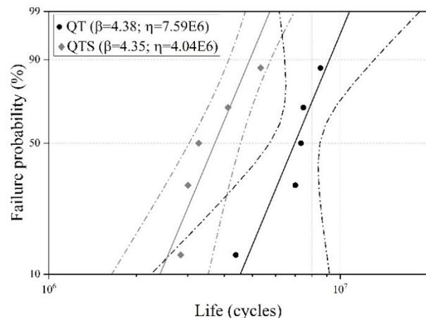
Figure 1: Failure probability curves for QT and QTS groups of specimens. Confidence interval: 90%.
