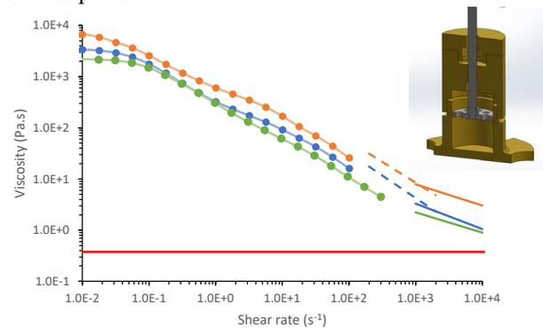
Figure 1: Viscosity as a function of shear rate and amount of degradation, rheometer measurement (circles), grease worker standard holes (dashed line) and small holes (solid line) and base oil viscosity (red line). Inset: grease worker
