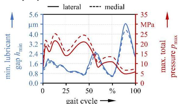
Figure 1: Minimum film height and maximum pressure evolution in the soft-EHL contact in TKRs during one gait cycle.
