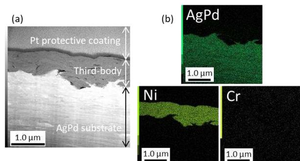
Figure 1: (a) STEM micrograph of the AgPd cross section showing the presence of a third body, (b) the corresponding EDS mapping showing that the third body is composed of Ni only
