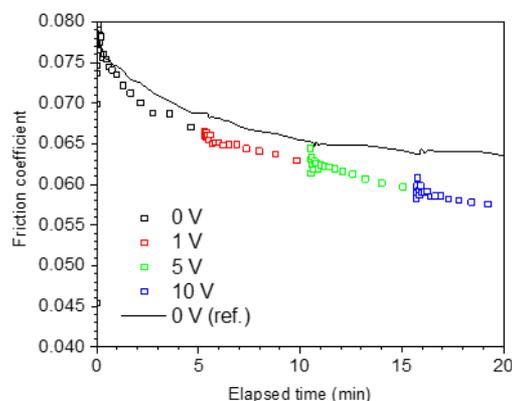
Figure 1: Evolution of the friction coefficient with time in a sequence of 4 consecutive steps with increasing electric potentials up to 10 V.
