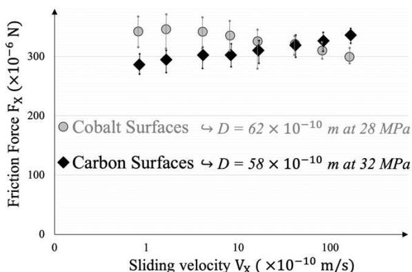
**Figure 1 :** The friction force  $F_x$  against the sliding velocity  $V_x$  for the Glyceryl Oleate adsorbed boundary layers on both surfaces, after running-in friction cycles.  $D$  = Interface thickness.
