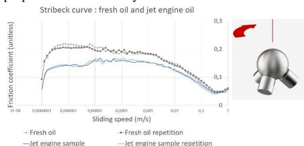
Figure 1: Stribeck curve for fresh and used lubricant samples, obtained with a BO3P system.
