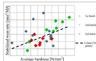
Figure 1: Correlation between wear rate and hardness.
