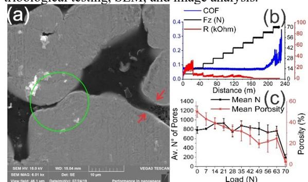
Figure 1: (a): Impregnated pore being sealed by the tribological process, (b): Evolution of COF as a function of load and distance, and (c): Evolution of the number of pores and porosity as a function of load.
