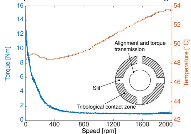
Figure 2: Results of the four slits sample at 2 MPa load
