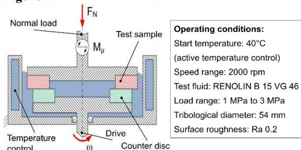
Figure 1: Schematic drawing of the test bench[1],[2]
