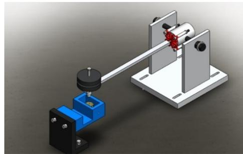
Figure 1: Schematic diagram of linearly reciprocating tester.
