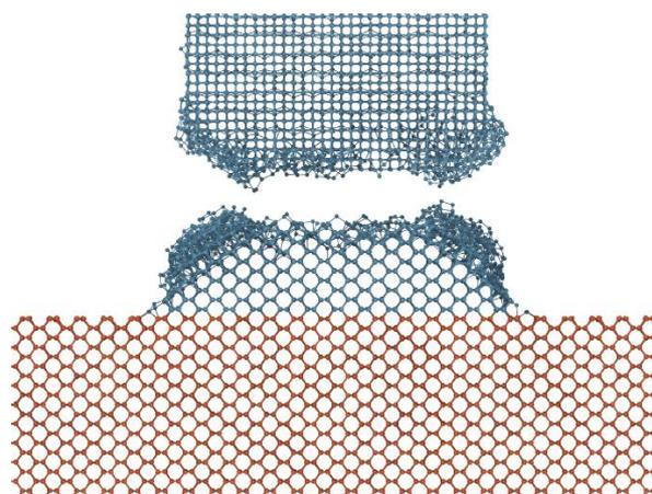
Figure 1: Triboepitaxial growth on an extended Si substrate in contact with a single asperity after sliding and subsequent lifting off the asperity. The color of the atoms refers to the crystal they belonged to prior to sliding (red substrate, blue asperity).
