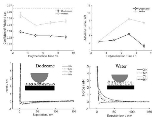
Figure 1: (top left) – friction coefficient data relative to bare silicon surface (dotted line). (Top Right) – Adhesion force data. (Bottom) – Force curve plots in dodecane (right) and water (left).
