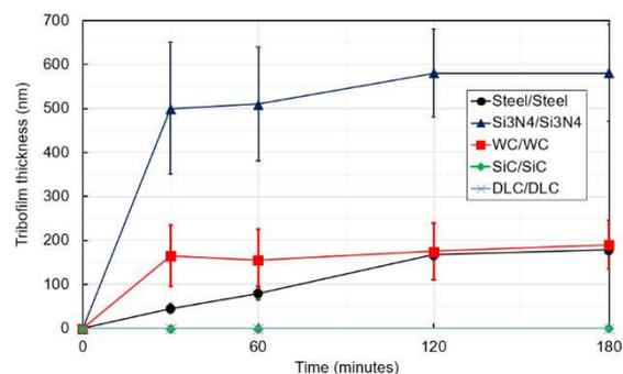
Figure 1. The evolution of ZDDP tribofilm thickness on each material during rubbing in thin film conditions.
