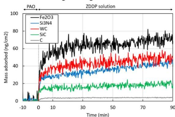
Figure 2. The evolution of ZDDP tribofilm thickness on each material during rubbing in thin film conditions.
