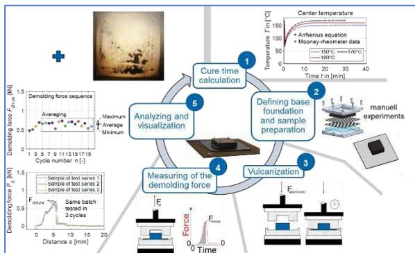
Figure 1: Vulcanization and Demolding process at the demolding test rig with parameter analysis and fouling evaluation
