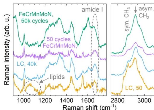
Figure 1: Raman spectra of accumulated wear debris of LC-CoCrMo and FeCrMnMoN pins measured after different numbers of cycles.
