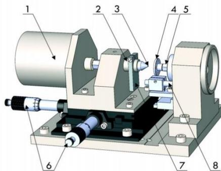
Figure 1: Figure 1: Impact Tester scheme: 1- inductor, 2- head, 3- indenter, 4- holder of sample, 5- force sensor, 6- micrometer screws, 7- mirror, 8- displacement sensor.
