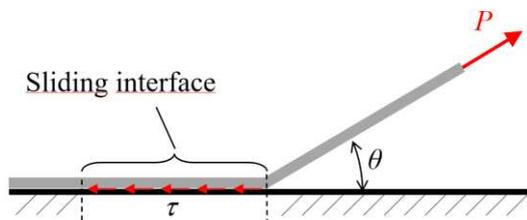
Fig1: Scheme of the peeling for a viscoelastic tape in presence of interfacial sliding.
