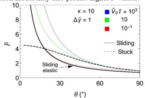
Figure 2: Comparison between dimensionless peeling load  $\tilde{P}$  for stuck and sliding model at different values of the parameter  $\tilde{V}_0 \tilde{\tau}$  for a fixed value of dimensionless energy of adhesion  $\Delta\tilde{\gamma} = 1$  and viscoelasticity parameter  $\kappa = E_\infty/E_0$ .
