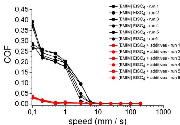
Figure 1: Stribeck curves of [EMIM]EtSO<sub>4</sub> and the additivated lubricant. Ramp test: decreasing sliding speed from 200 mm/s to 0.1 mm/s. Normal load 4.5 N. radius 8 mm.
