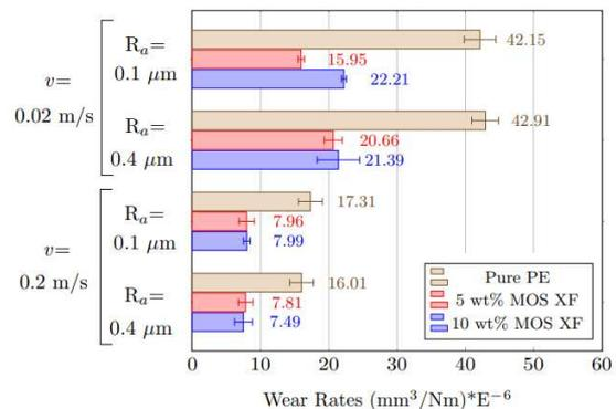
Figure 1: Wear rate of MOS XF reinforced UHMWPE.
