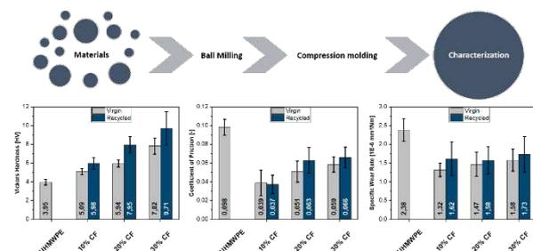
Figure 1 Manufacturing procedure, Vickers hardness, coefficient of friction and specific wear rate of UHMWPE/CF composites.
